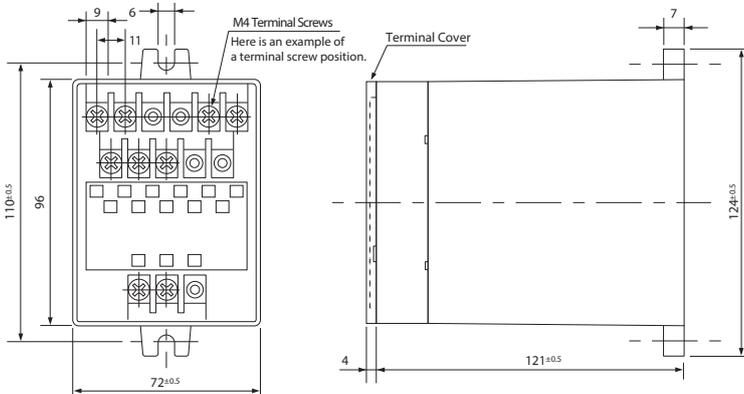
**Case Material: Glass fiber-strengthened PC resin**
