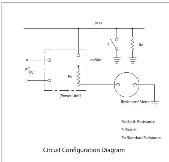
Apply an AC power supply to the extra power unit to generate DC50V on the output side. This DC power supply can be used to combine the unit with a DC ammeter with an M $\Omega$  scale, making it possible to take measurements and read earth resistance for circuit currents that change depending on the ground status.
