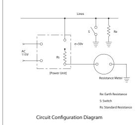
Apply an AC power supply to the extra power unit to generate DC50V on the output side. This DC power supply can be used to combine the unit with a DC ammeter with an M $\Omega$  scale, making it possible to take measurements and read earth resistance for circuit currents that change depending on the ground status.
