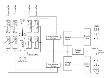
Wide-angle Meter Relay Photoelectric-type Circuit Configuration
